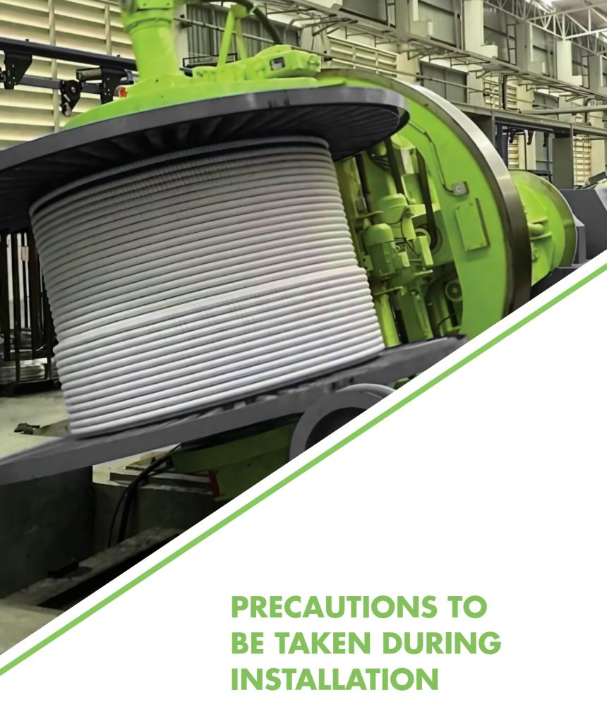
Never lay the drum in flat position & never pull the cable from such flat laid cable drum.
