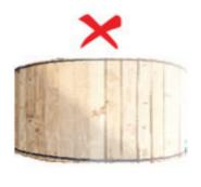
Do not lay drums flat on their sides, use proper wedges to prevent drums rolling.
