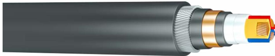
ii) Oman Cables have the capability to manufacture low voltage grade cables with copper tape screen and interstitial bare conductor(s). The size of the interstitial conductor(s) shall be equal to half of the phase conductor. Interstitial conductor(s) can be one or three, depending upon the requirement.
