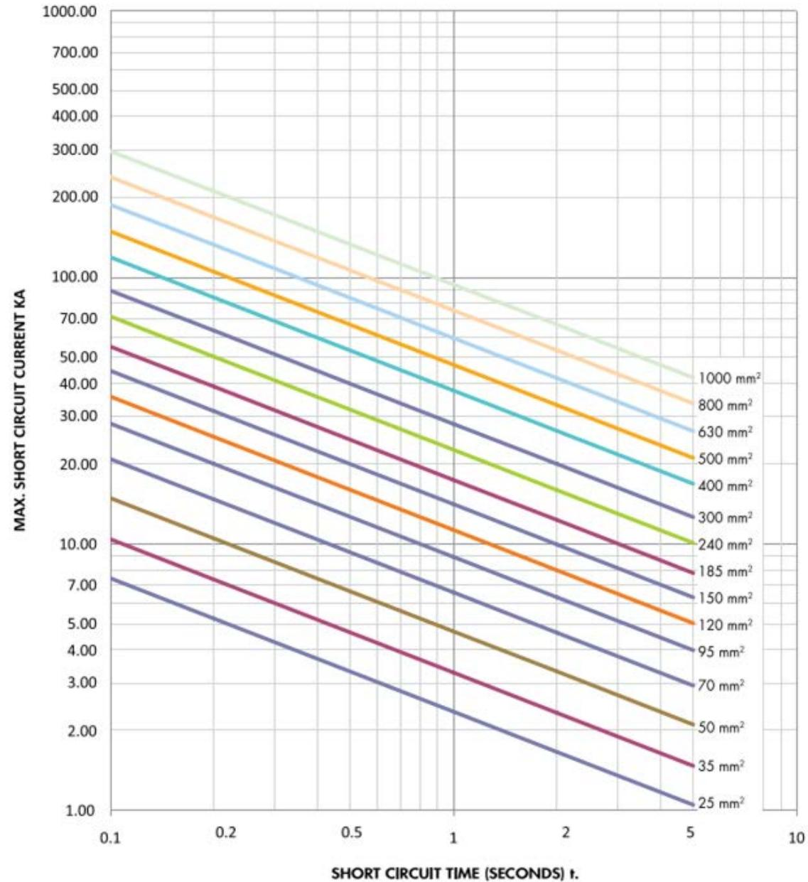
For PVC insulated cables, the short circuit current rating for copper conductors is calculated by the formula mentioned above, while considering the continuous operating temperature as 70 °C and the short circuit temperature as 160 °C up to 300mm<sup>2</sup> and 140 °C for sizes above this.
