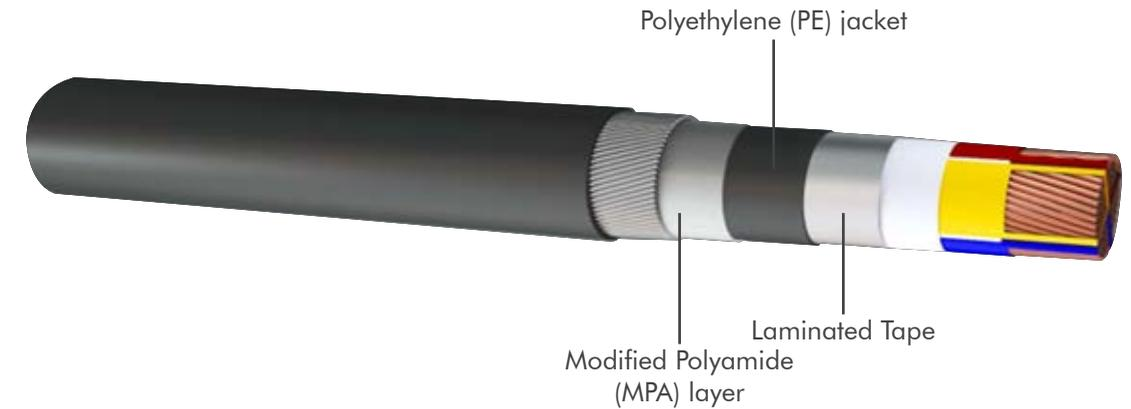
Typical constructional diagram for Multi Core Copper DRYLAM Armoured LV Cable
