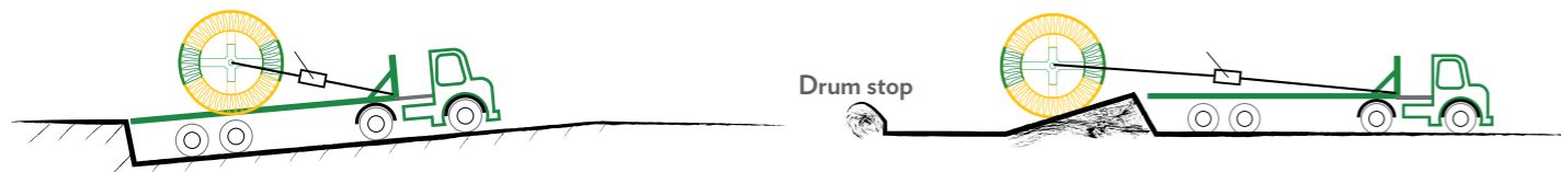
Method 1: Hole excavated (Maximum slope 1 in 10) to receive truck.
